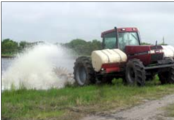
Figure 15. Tractor powered (PTO) "sidewinder" type paddlewheel aerator.
