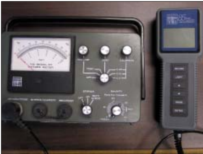
Figure 10. Commonly used electronic oxygen meters.
